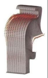
Reaction forces in the uplift restraint of Alternativ I
